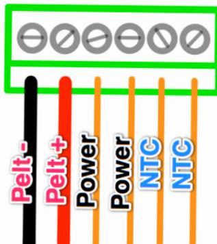
Use your 2 mm screwdriver to loosen the terminals (righty tighty lefty loosey). Hold each
