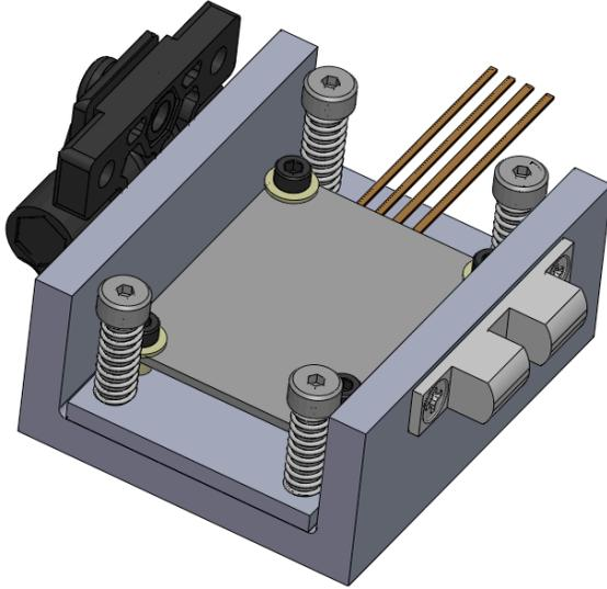
There are 4 wires coming out of the lid heater. 2 are labeled “NTC”. 2 are labeled “Power”. These labels are very important. If they get mixed up, the heated lid may break the first time it is plugged in.
