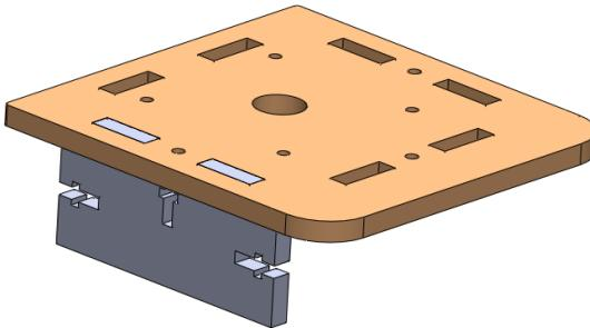
Pick up a small metal nut. Slide the nut into the “t” cross of the Side piece as shown. (Line up the edges of the nut to be parallel with the cross.)
