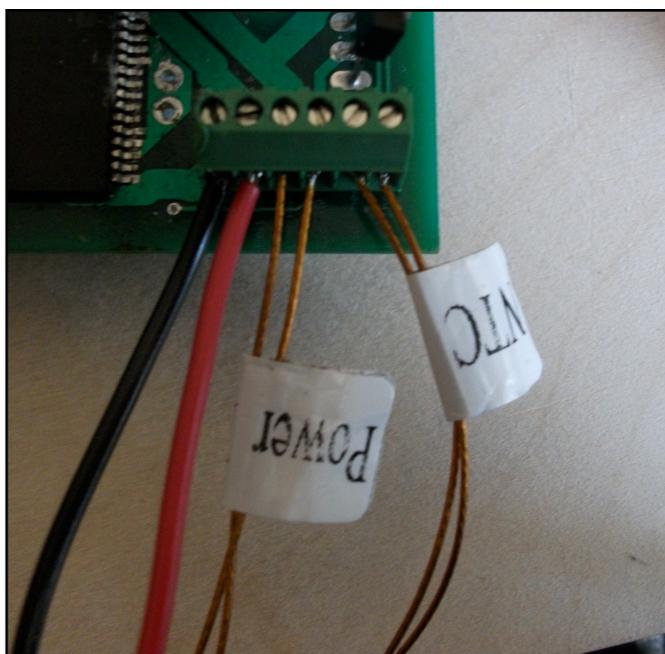
Connect the wires for the Lid Heater to the OpenPCR board. All 4 wires connect to the green terminal. The order is very important!
