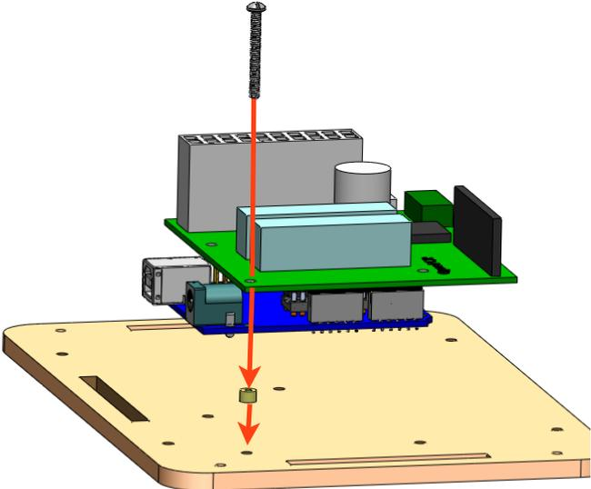
If you have needle nose pliers, use them to hold the spacers in place while you put the screws through.
