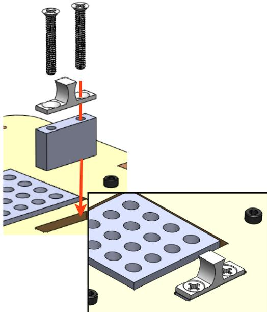
With the hinge block and 2 philips head screws, attach the heated lid. Close and open the lid. You may need to loosen the screws on the side of the latch that control the latch tension in order to open the lid easily.
