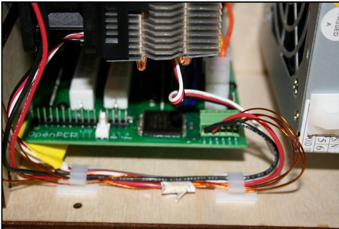
Clip the 4 tan lid heater wires + red and black peltier heater wires to the clip on the fan.
