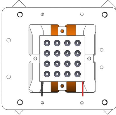
Find the 4 pieces of white insulation. The notched piece is for the block temperature sensor wire. Remove the backing from the white insulation strips and stick them to the sides of the block.
