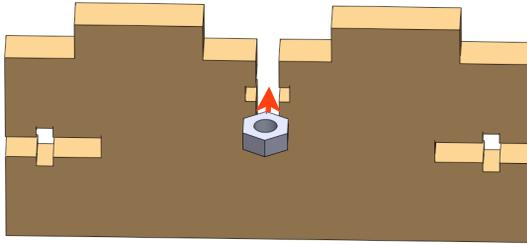
Put a metal screw through the hole as shown. Tighten it using your fingers at first. Finish it off with your blue Allen wrench.
