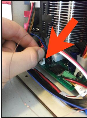
Wrap the heat block temperature sensor once
