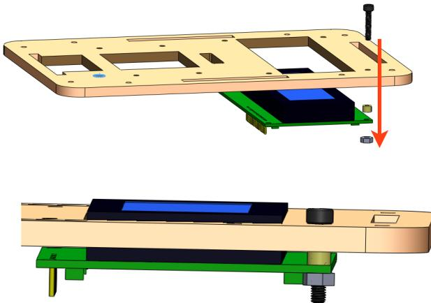
The LCD pins must be on the same side as the highlighted hole (blue)
