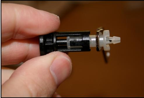
Find your pliers and break off 2 of the black plastic tabs. Avoid bending the metal arm. You can put the plastic parts in the trash.
