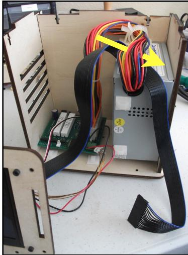
There's two wires remaining: one which connects to the the block temperature sensor, and the LCD cable. Leave them disconnected for now. Keep them away from the rest of the wires to make sure they do not snag or break.
