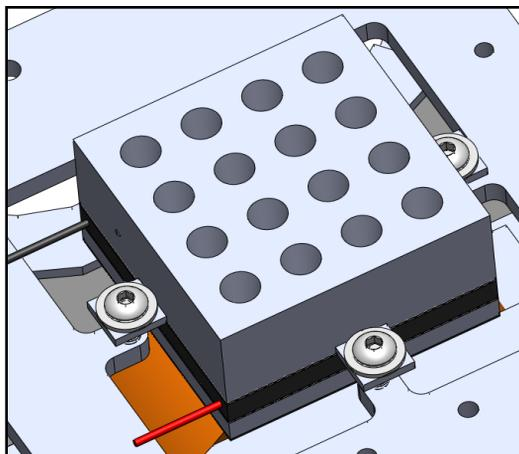
Check all the edges are aligned and no one part sticks out. Check the arms don't touch the mounting plate.
