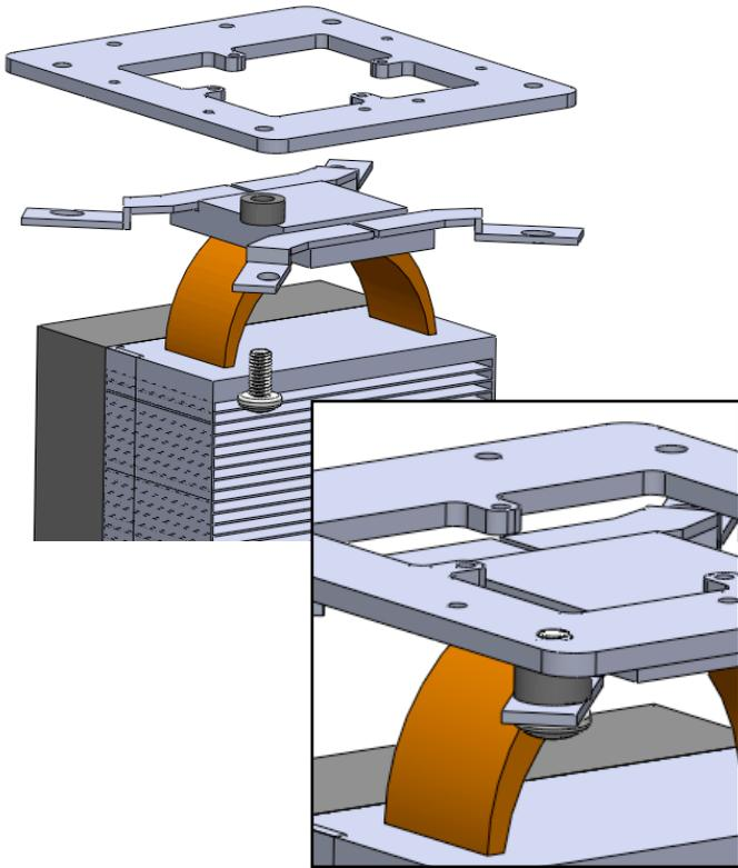
Repeat with the 3 other screws. Tighten the small screws on the heat sink arms, as well as the large screws. Don't over-tighten, stop if the arm starts to bend.
