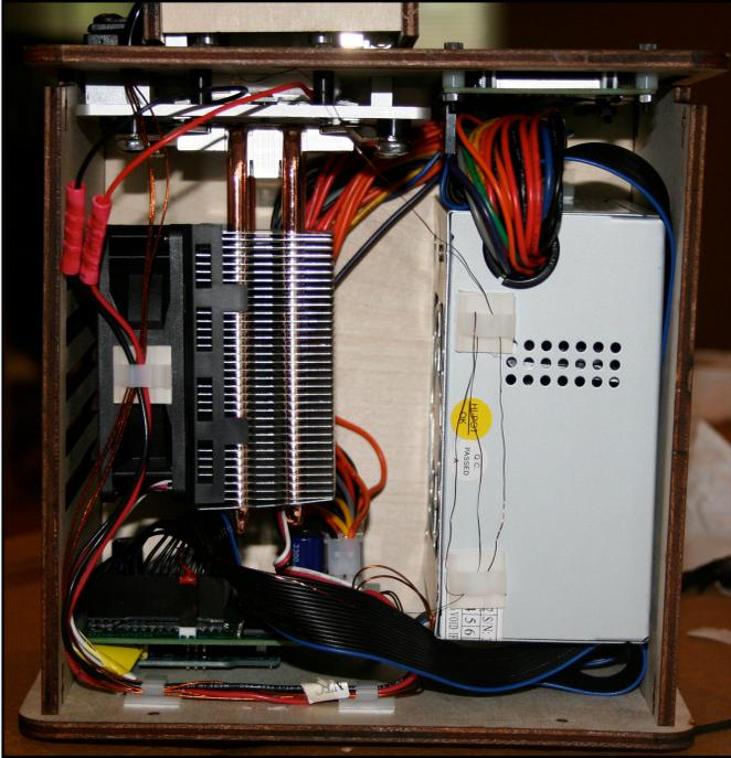
If the Power Supply wires are blocking the power supply fan, make sure to push them out of the way. The same applies to any other wires that might block OpenPCR's airflow.
