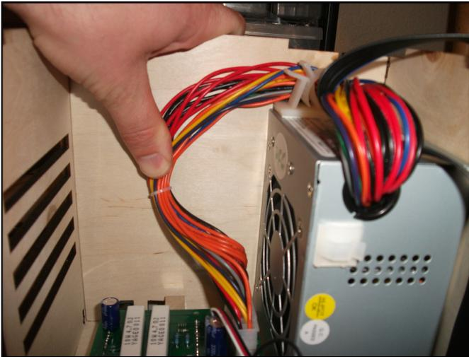
Make sure the Power supply cable does not block the power supply fan
