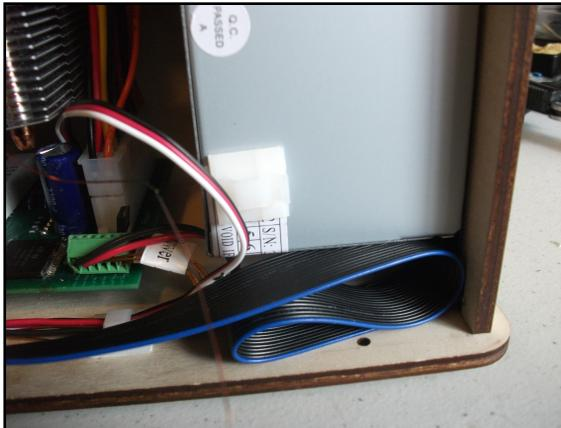
Plug in the heat block temperature sensor wire.
