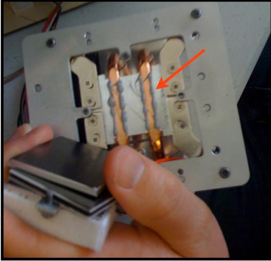
Stack the aluminum plate, peltier, and block with all thermal pads facing DOWN. **Red peliter wire must face RIGHT** as shown, where the fan is on the left!
