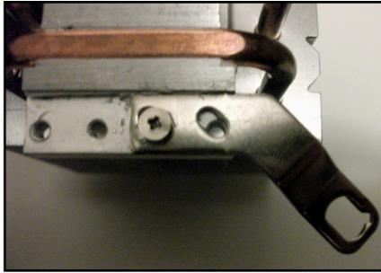
Repeat for the other 3 arms. Leave the screws a little loose, so the arms can wiggle a little bit. You'll tighten these in a few steps. Throw the other fan parts away, except for the thermal paste.
